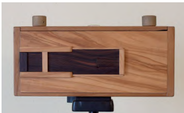
Camera Pinhole 6x12; 30mm, f/120
